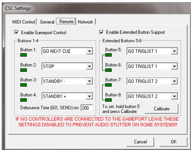
A standard MD Split cable will split the 4 fire buttons to a local remote control box for the operator (giving GO, STOP, PREV, NEXT) which will appear in CSC as buttons 1-4, and buttons 6 and 8 are wired to female XLR connectors which can be connected to a GO-STOP button in the pit, via the analogue multicore.
